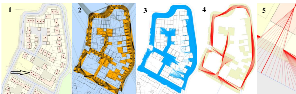
Figure 3 Finding R2D path using a visibility graph (Ordnance Survey © Crown copyright 2017)
